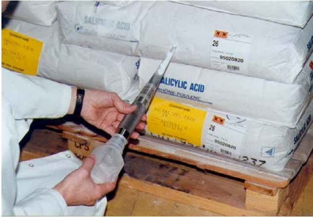
The sampling chamber collects the samples...
