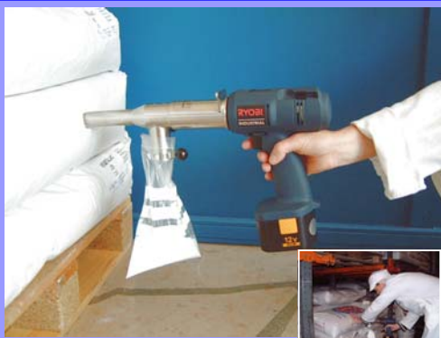
Horizontal sampling in a sachet from paper sacks on a pallet with a 300mm long sampler Ref. S6PH3R
