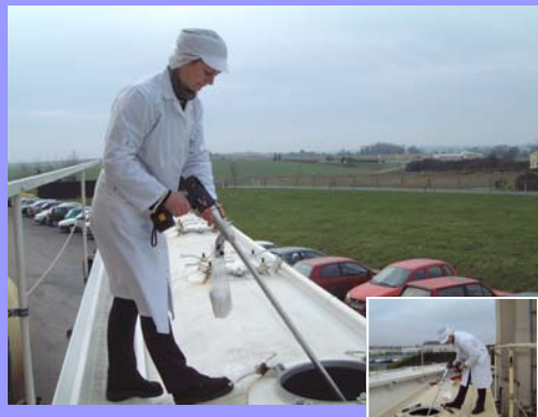
Vertical sampling in a sachet From bulk tanks with a 1500mm long sampler Ref. S6PV15R
