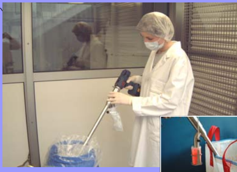
Vertical sampling in a sachet/bottle from drums or big-bags with a 600mm long sampler Ref. S6PV6R
